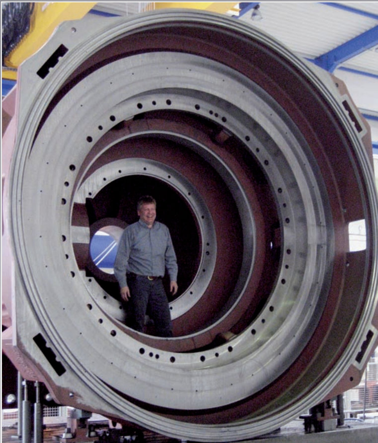
Transmission housing EN-GJS-500-7, finish machining \varnothing 2164 mm and \varnothing 2335 mm, V_c : 170 m/min, cutting depth: 0.5 mm, f_z : 0,10 - 0,12 mm
